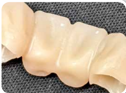
Figure 2. White spots on the outside of zirconia crowns.
