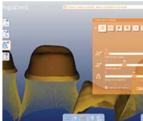
Image 21. (above) Setting the Die Spacer and Coverage
